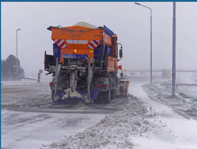
A snowplow clears snow while simultaneously spreading salt on the road. Photo from Watersheds Canada
